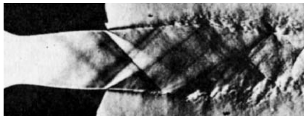
(d) p_G/p_2 = 1.37 . External pressure less than pressure inside nozzle (nozzle under-expanding). Fans of expansion waves formed at edges of nozzle exit, through which pressure is lowered to ambient value. Jet diverges and expansion waves are reflected from opposite surface as compression waves. Hence diamond pattern in which alternate expansion and compression continue until damped out by viscous action.
