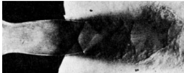
(c) p_G/p_2 = 0.85 . Nozzle still over-expanding; external pressure lower than in (b). Oblique shocks now weaker; they cross jet and are reflected from opposite surface of jet as fans of expansion waves. This is because boundary condition at edge of jet is not unchanged direction (as at a solid boundary) but unchanged pressure. Pressure rise through incident shock wave can be cancelled only by an expansion. Hence diamond pattern in which alternate compression and expansion continue until damped out by viscous action.
