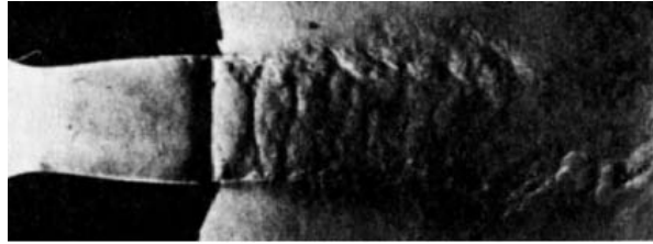
(a) External pressure greater than pressure for isentropic flow throughout nozzle (nozzle over-expanding). Normal shock wave just inside nozzle.
